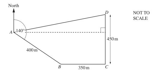
The diagram shows a field ABCD. The bearing of B from A is  $140^{\circ}$ . C is due east of B and D is due north of C. AB = 400 m, BC = 350 m and CD = 450 m.
